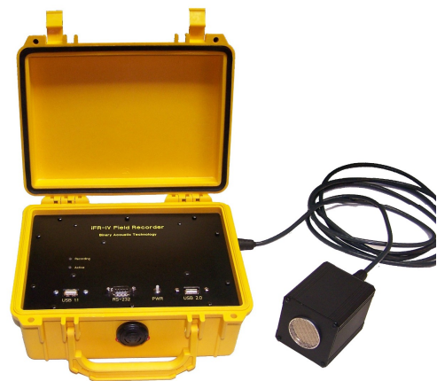
iFR-IV with ultrasonic microphone
