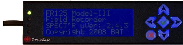
The LCD controller is an optional module that simplifies iFR-IV configuration and operation. The LCD controller is a standalone module that plugs into one of the iFR-IV USB ports. It consists of an LCD character display along with six push buttons; up, down, left, right, enter and exit.
